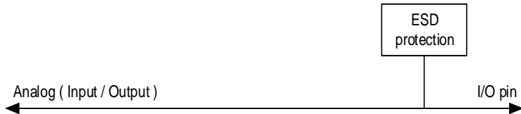
Figure 7-4. Basic structure of Analog configuration
